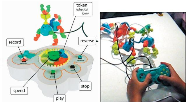
Figure 1: *Remix*, left, is a tangible sampler/sequencer for *Topobo* robotic construction toys, back. A child uses the *Robo* controller, right, to outperform his friend’s creation in a “battle-bot” competition.
